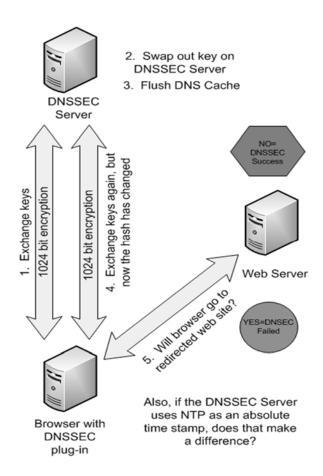
*Figure 4*. Drawing of the Experiment Design. The experiment begins with a successful MiTM attack. A DNSSEC-enabled browser attempts to go to a redirected web site. This is done with and without NTP influencing the TSIG field of the DNSSEC Server.
