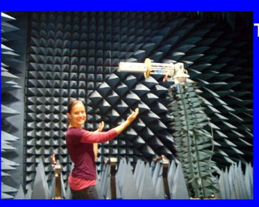
Testing in anechoic chamber of FirstRF Corp. to determine the antenna gain pattern →
