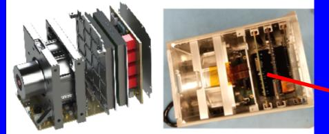
REPTile-2 fully integrated and tested (plus a spare copy – for post flight calibration)
