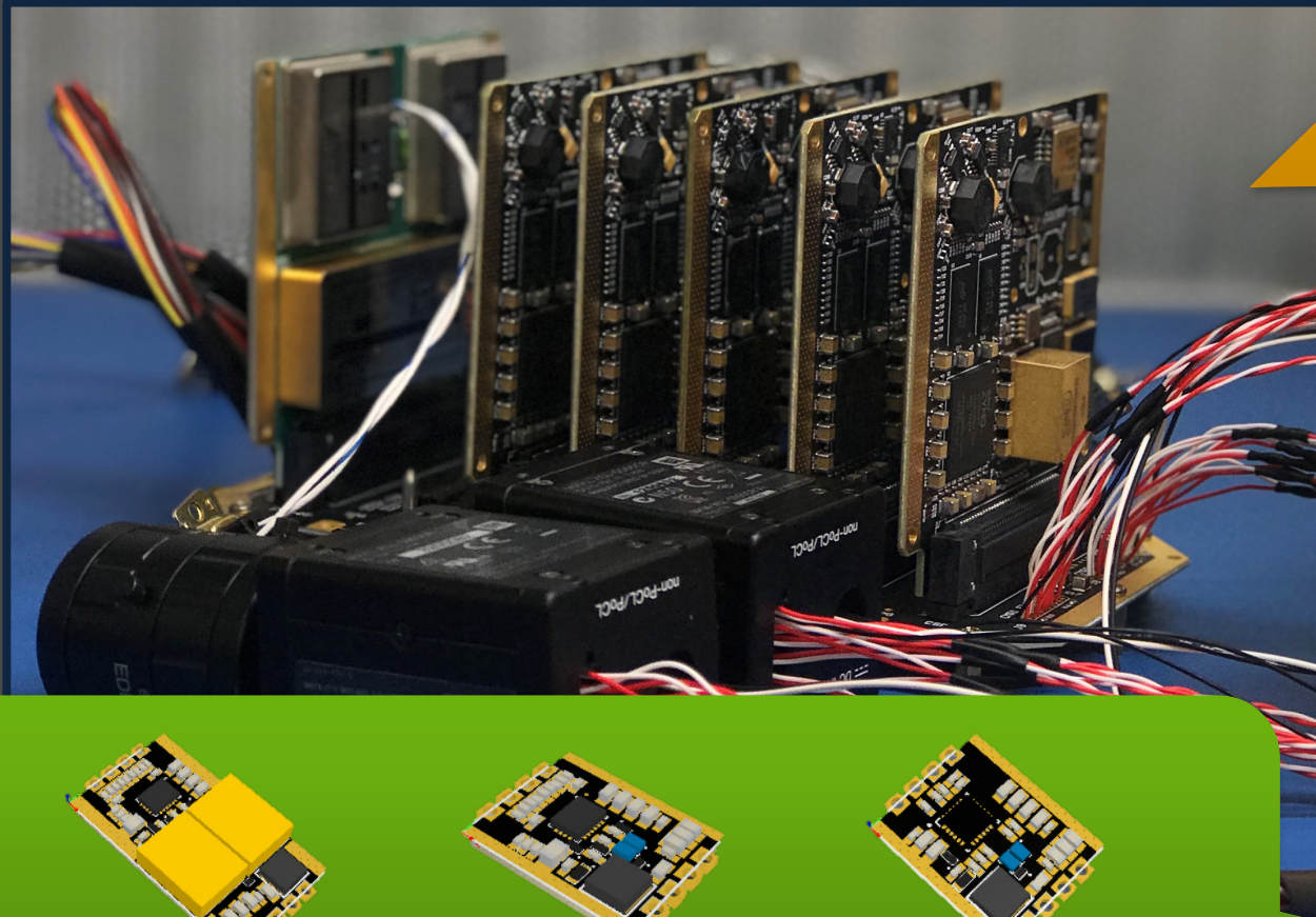
Gallium-Nitride (GaN) Point-of-Load (PoL) Converter Experiment
