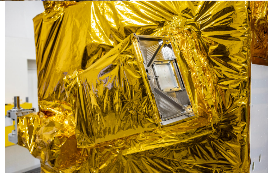
Final Closeout of LICIACube Thermal Blankets Prior to Launch
