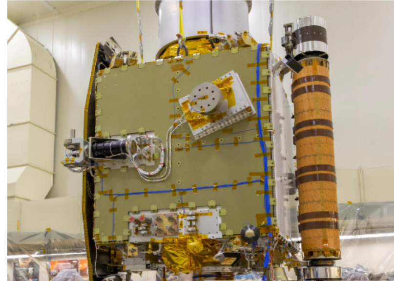
LICIACube Mass Simulator Mounted on the DART Spacecraft during Vibe Testing
