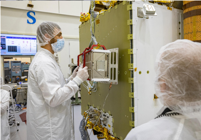
Installation of Flight LICIACube Assembly on DART Spacecraft
