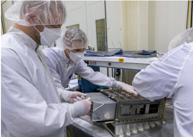
Stowing of Thermal Simulator into Dispense in Preparation for TVAC Testing
