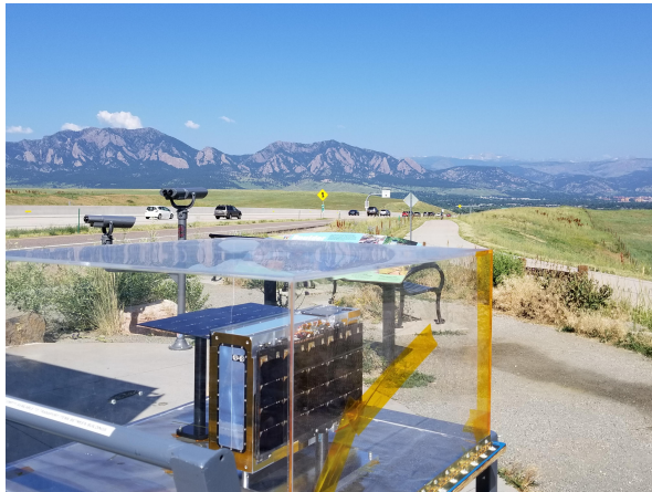
Figure 8: The outdoor radio test. CUTE is mounted inside a polycarbonate box to protect it from dust and pollen. The single solar panel is deployed to free the UHF. The S-band antenna is aimed at the LASP ground station. The Flatirons are in the background.
