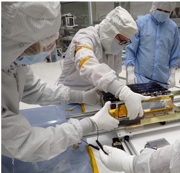
Figure 9: Two CUTE team members (left and center) place the CUTE spacecraft on the conveyor to be installed in the PSC canister in Vandenberg Space Force Base.
