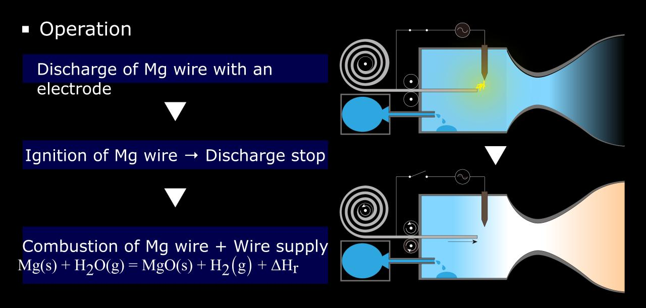
Verification of Mg-wire combustion in water vapor flow
