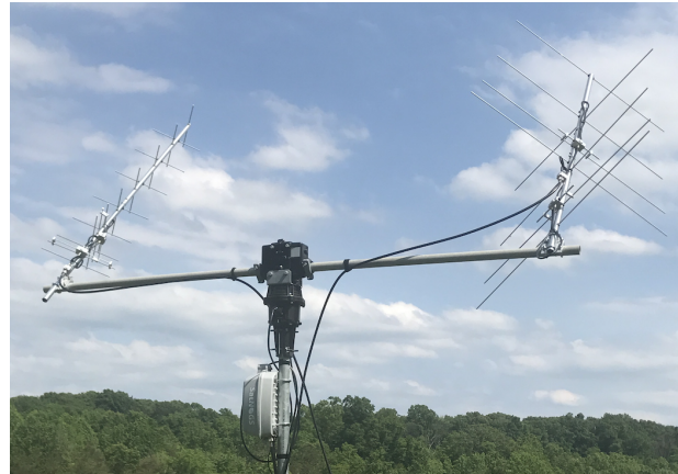
Figure 15: Corey Shields KB9JHU ground station #2 with commercial rotator with UHF and VHF antennas.
