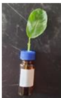
Figure 4.1 Alfalfa leaf setup for photodegradation experiments. For actual experimental samples, the leaf stem was pushed deeper into the vial so the leaf was positioned closer to the cap of the vial. This ensured a stable positioning of the leaves for the duration of the experiment.
