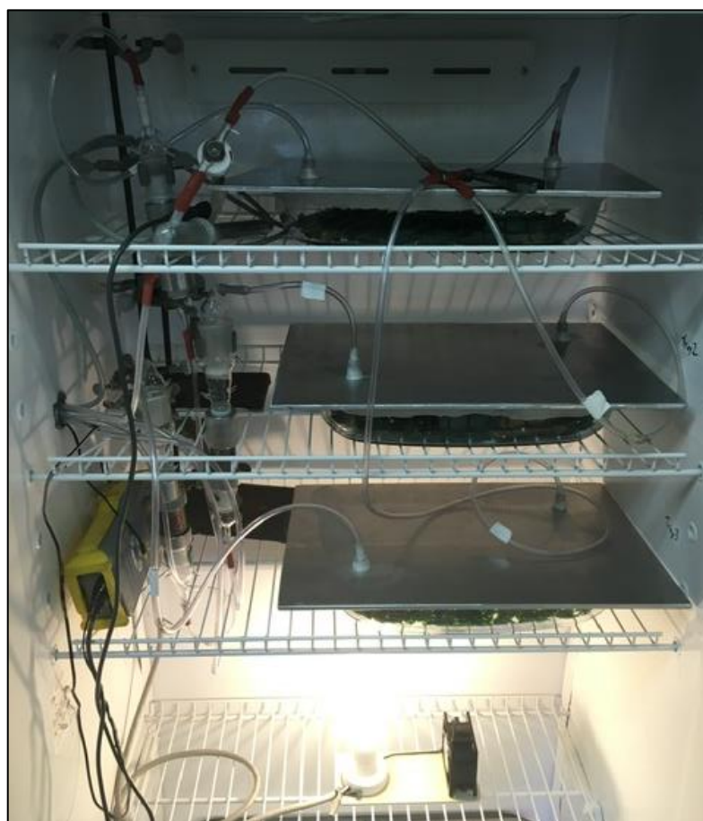
Figure 3.2 Photograph of inside the solid-phase fugacity meter.
