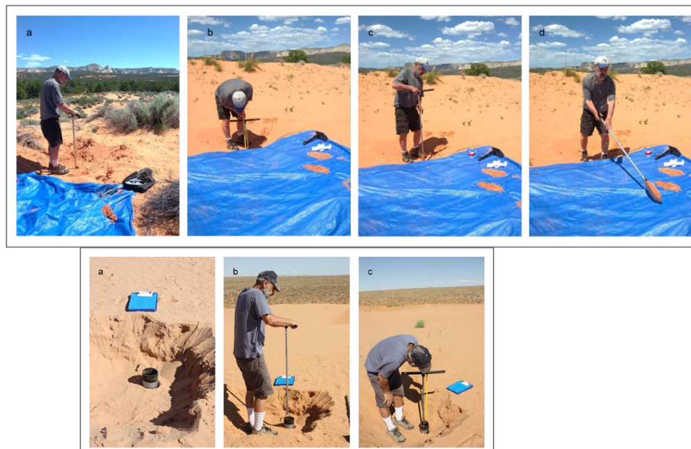
Figure SM-2.1 Sediment sampling with auger. Row 1 shows extraction of sediment sample, moist dune soil, from cleared platform base, Kanab, UT: a) starting auger hole; b) measuring depth to sample; c) careful vertical extraction, avoiding sidewall disturbance; d) emplacing sediment sample for geologic description and sample collection. Row 2 shows use of PVC collar with cleared platform in dry dune soil conditions, San Rafael desert, UT: a) platform cleared, collar emplaced for measurement with duct tape; b) starting auger hole; c) measuring depth to sample.
