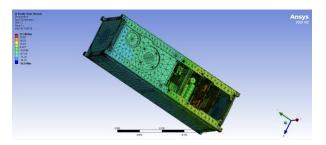
Figure 13: ANSYS steady-state thermal simulation results for sunlit case
