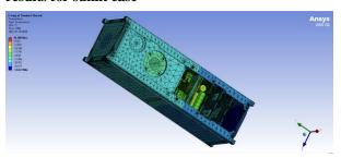
Figure 14: ANSYS transient thermal simulation results for eclipse case
