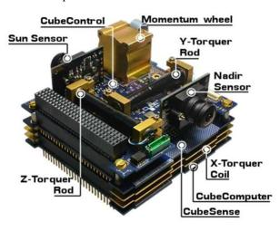
Figure 6: CubeADCS Y-momentum COTS system from CubeSpace, from datasheet
