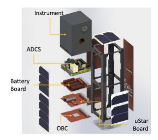
Figure 5: Exploded view of 3UCubed CAD model
