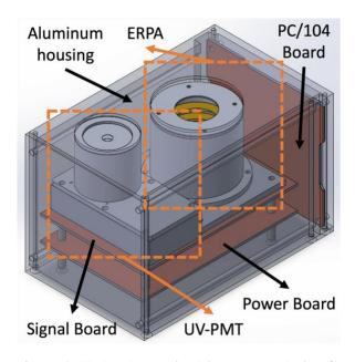
Figure 1: Updated combined instrument design for 3UCubed
