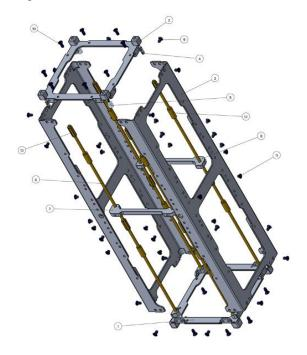
Figure 12: Exploded view EnduroSat 3U Structure, from datasheet
