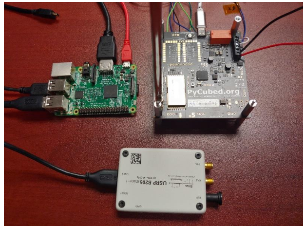
Figure 5: Picture of main components of NASB bus with SDR Payload
