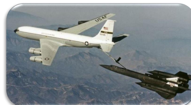
Figure 5: Example of in-air refueling (Graham 2013)
