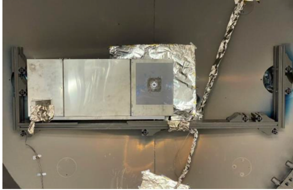
Figure 7: ENPULSION NANO R 3 propulsion system mounted to the FOTEC direct thrust test stand 25
