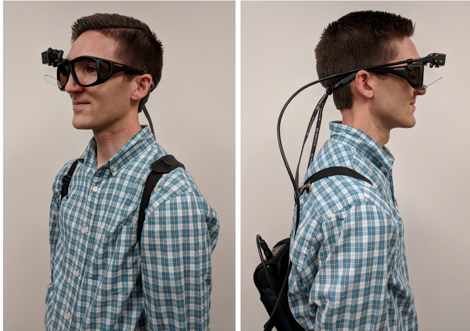
Fig. 6: An example of a subject wearing the ETMOBILE eye-tracking device. The eye tracker has one forward facing camera and one infrared camera that tracks the eye's movement by use of a transparent mirror.
