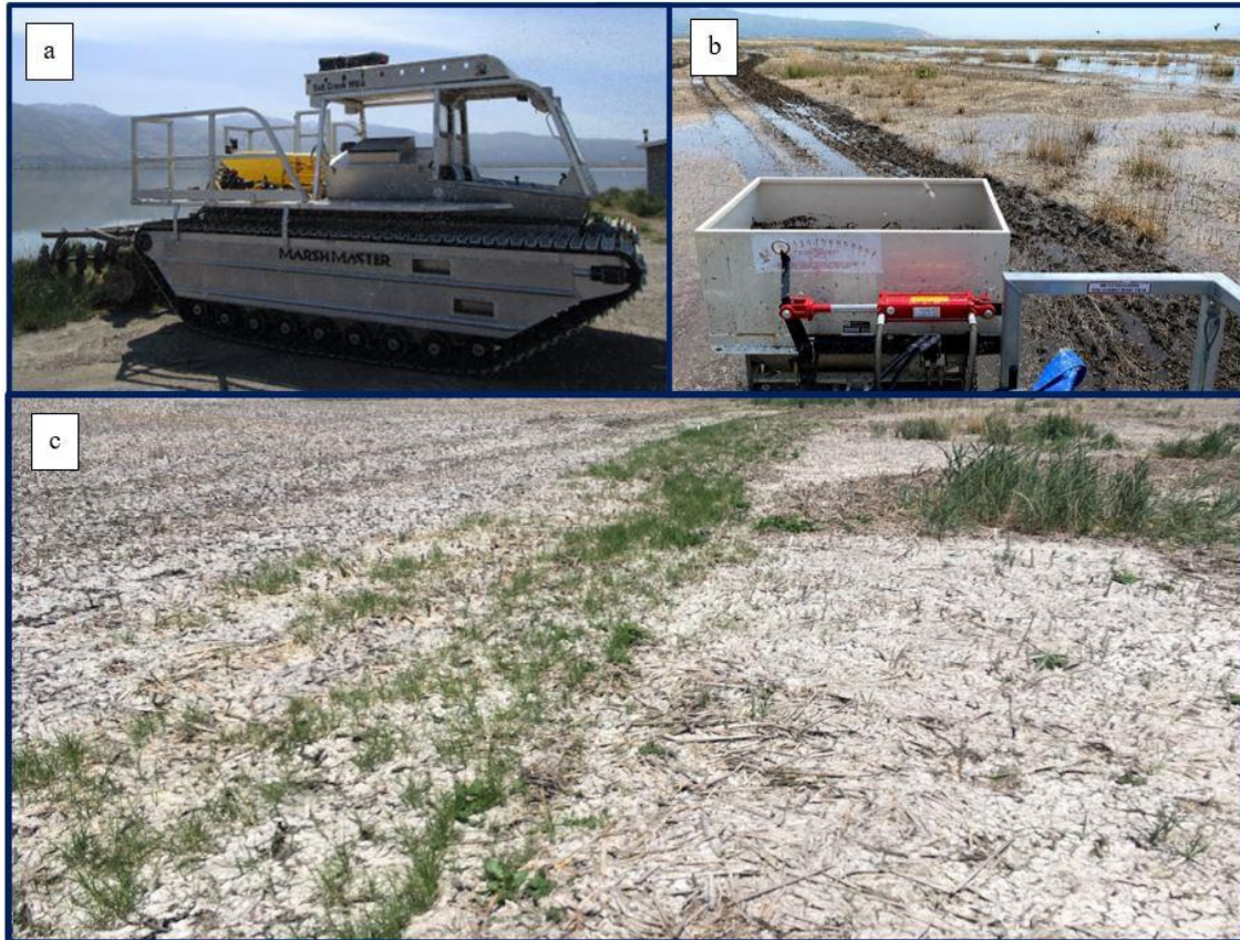
Figure 2.3. (a) The Marsh Master with an attached disc roller; (b) example of broadcast seeding method where machinery was driven adjacent to disced areas and (c) alkali bulrush germination in ruts created by disc roller (Field experiment 2021).
