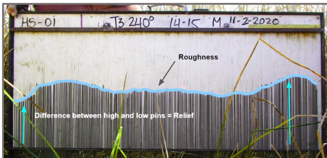
Figure 3.3. A profilometer was used to measure microtopography shown here with examples of roughness and relief.
