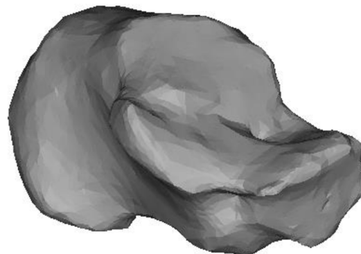
Figure 7. The anatomical CAD model created from CT imagery in the Mimics software.
