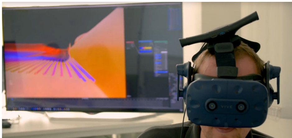
Figure 4.19: HTC VIVE Pro VR headset with wireless adapter
