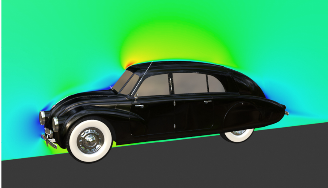
Figure 1.15: The visualization of the computational fluid dynamics using the Covise editor and the cutting surface node in Blender
