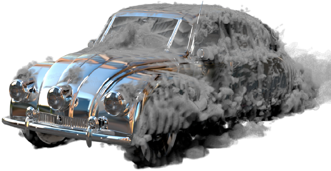
Figure 1.16: The volume rendering of the computational fluid dynamics using the Covise editor and the isosurface node in Blender
