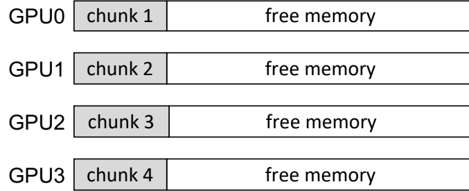
Figure 3.16: The first way of allocation of data structure in the Unified Memory of the multi-GPU system: Fully distributed data structure
