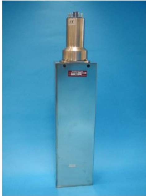
Figure 7.2: NaI(Tl) Spectrometer produced by Scionix Holland.
