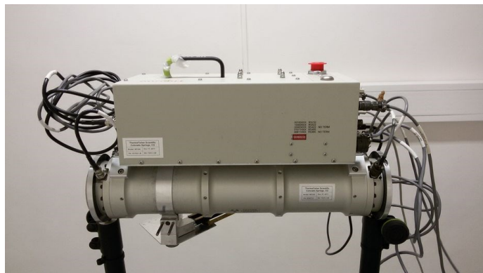
Figure 7.1: MP320 D-T Neutron Generator used at VŠB-TU Ostrava.
