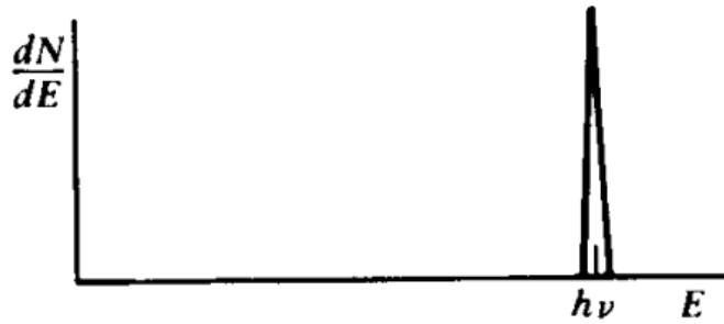
Figure 4.1: Distribution of energy given by photoelectric absorption.
