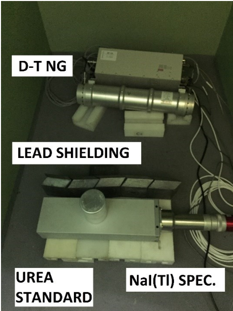
Figure 7.5: Placement of components at Department of Nuclear Reactors in Prague.
