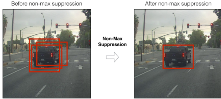
Figure 2.14: Before and After of Non-Max Suppression [23].
