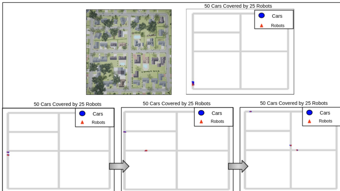
Figure 6.4: Multi-Robot Coverage On the top, the figure on the left represents a top down view of our environment in which we test our robots. Targets are constrained to move on the road while robots are free to move anywhere 5 meters above the ground plane. On the bottom, we visualize the behavior of the robots over time (left to right) and observe the robots are able to split up and cover the targets even when the robots have not been trained to cover splitting behaviors in the targets.
