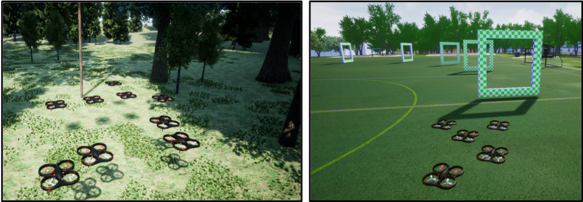
Figure 5.1: Learning Decentralized Perception Action Communication Loops for Robot Teams. Relying only on onboard visual and inertial sensors, robots compute decentralized control policies to fly through the constrained environment.
