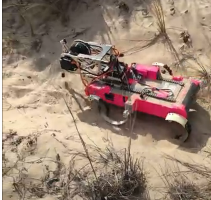
Figure 2.3: RHex carries a payload and walks along a human trail up and down the crests of multiple dunes to reach a study site in Oceano Dunes in 2016. The hike lasted 17 minutes, after which the robot continued to operate for another hour as it was used to take samples. It was able to make these repeated ascents in large part due to the increase in gearbox ratio from 28:1 to 79:1.
