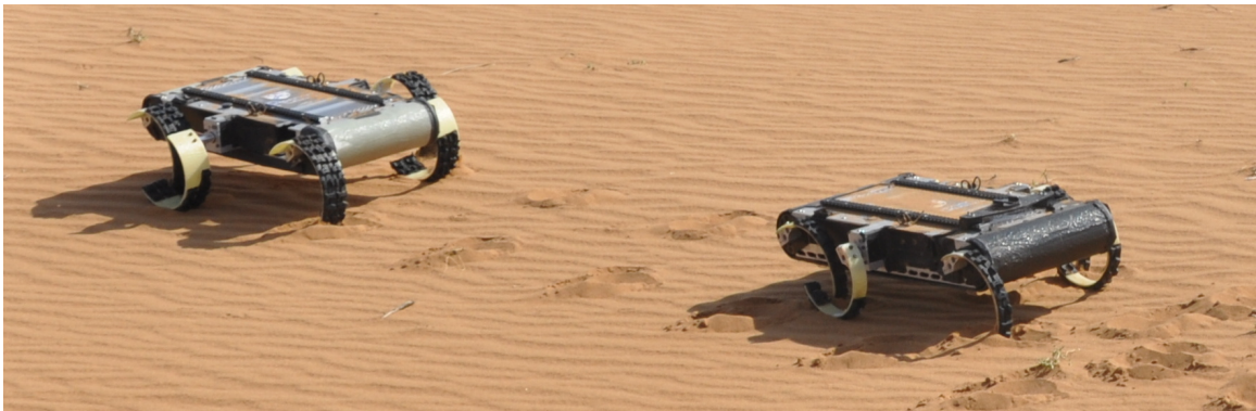
Figure 2.2: Specific resistance experiment in which the two robots walked together for 30 minutes over the same territory [110].
