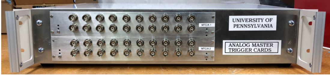
Figure 37: The front panel for the MTC/A chassis. The chassis contains two MTC/As, each with 20 analog inputs.
