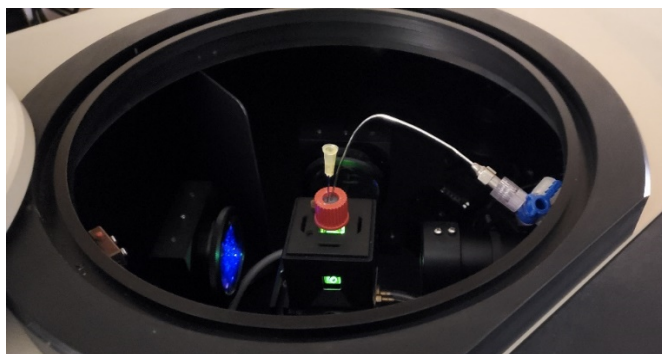
Figure 5.10. The photoredox reaction set-up. The reaction mixture was irradiated at 406 nm under an atmosphere of Ar (g) at 23 °C.
