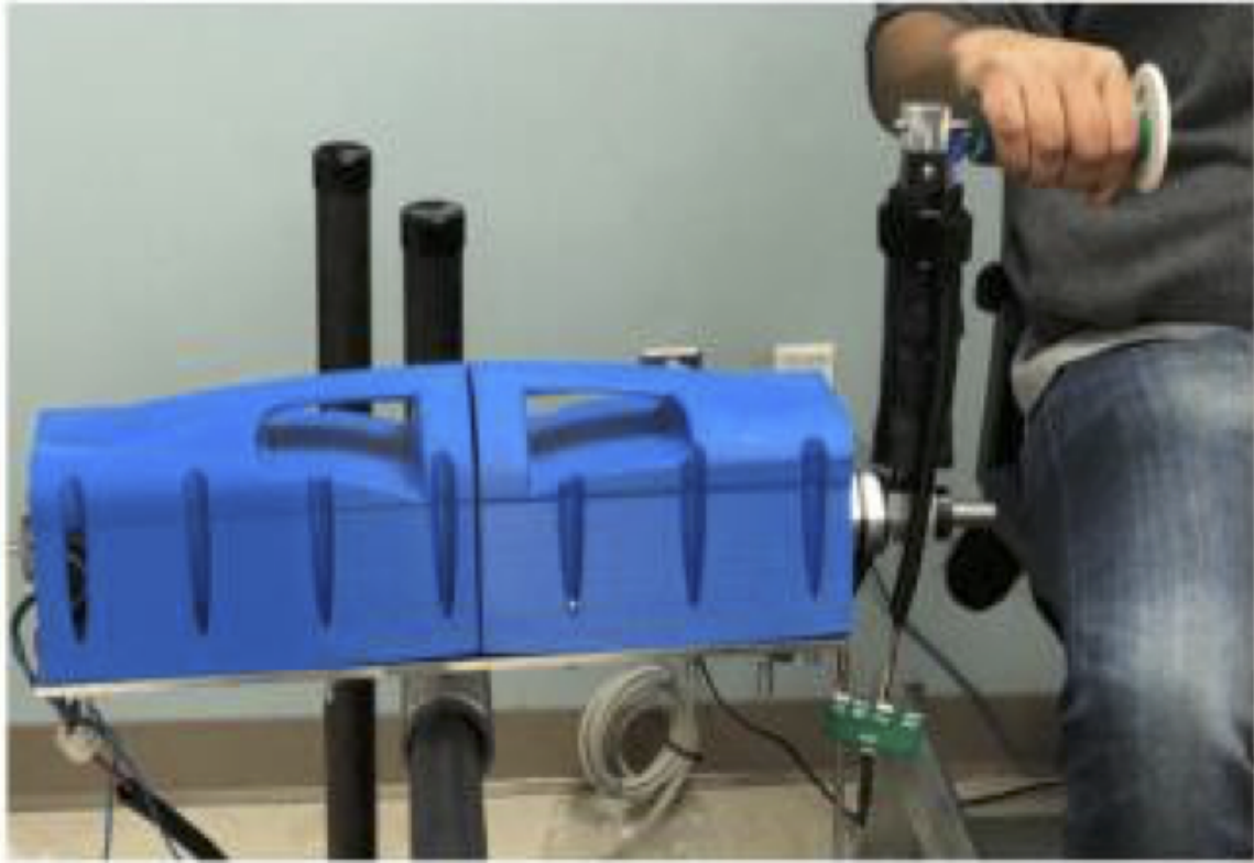
Figure 6: The Haptic Theradrive, a one degree-of-freedom rehabilitation robot system used in this study. Image used with permission from (Bui et al., 2017).
