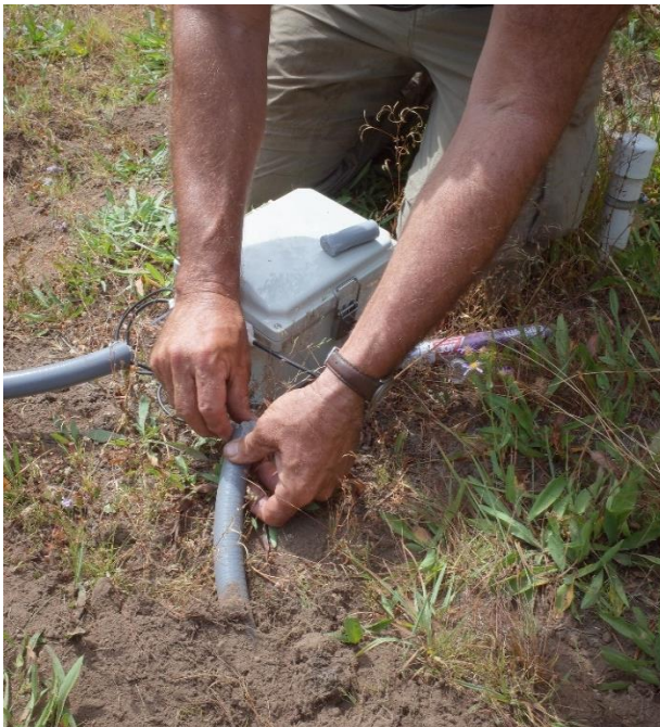
Figure 3.10. Top Left - snowpack nearly covering the weather station in Miranda Cabin Meadow, winter 2017, Top Right - damage to weather station following deep snowpacks, Bottom Left - protective conduit being installed on sensor cables, Bottom Right - water within water-proof box housing data loggers.
