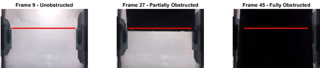
Figure A-1. Still shots extracted from iPhone footage for use in the camera calibration process.
