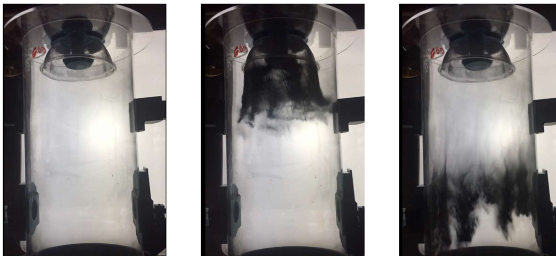
Figure 3-5. Snapshots of the powder cloud forming in the vessel. The powder was ejected from the dust dispersion system and then fell to the bottom collection pan.
