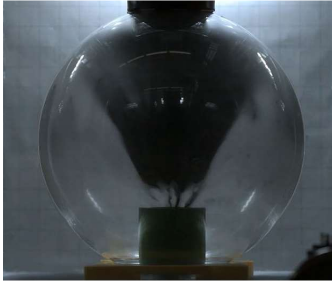
Figure 1-4. Transparent replica of ANKO 20L spherical apparatus for highspeed filming of the cloud.
