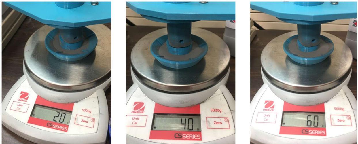
Figure A-4. Different amounts of powder in probe trials: 20g, 40g, and 60g.
