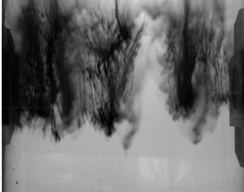
Figure 4-2. Snapshot of the cloud falling through the vessel, displaying the tendency of the powder to fall in plumes. This demonstrates the lack of uniformity within the powder cloud.
