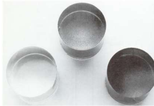
Figure 2-8. Epoxy samples experimented with for probe calibration in the Three Probes study [7].
