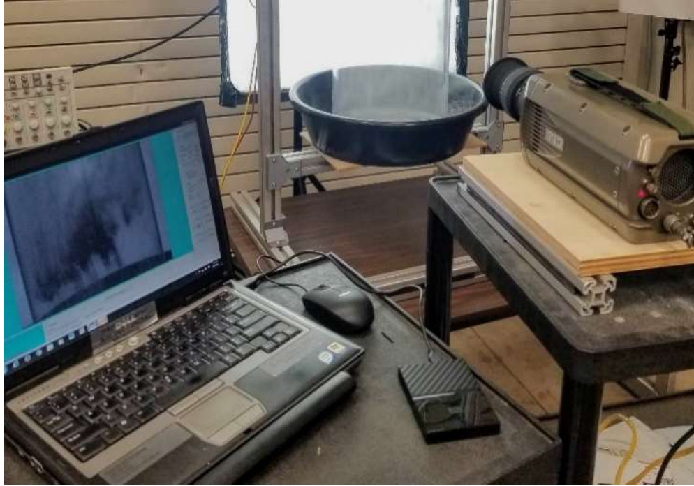
Figure 3-7. Phantom highspeed camera setup.
