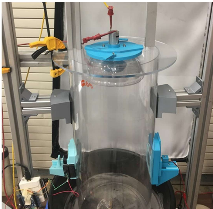
Figure 3-4. Full dust dispersion assembly, as used in situ.
