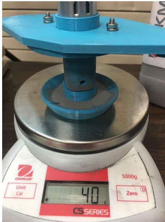
Figure 3-6. Weighing out 40g of tungsten powder for each sample.
