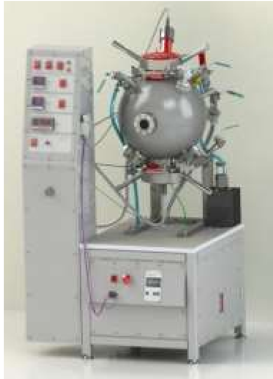
Figure 1-3. The ANKO 20 Liter explosibility test apparatus is one of several devices recommended in ASTM E1226 to determine the risk of deflagration for a dust sample [5].
