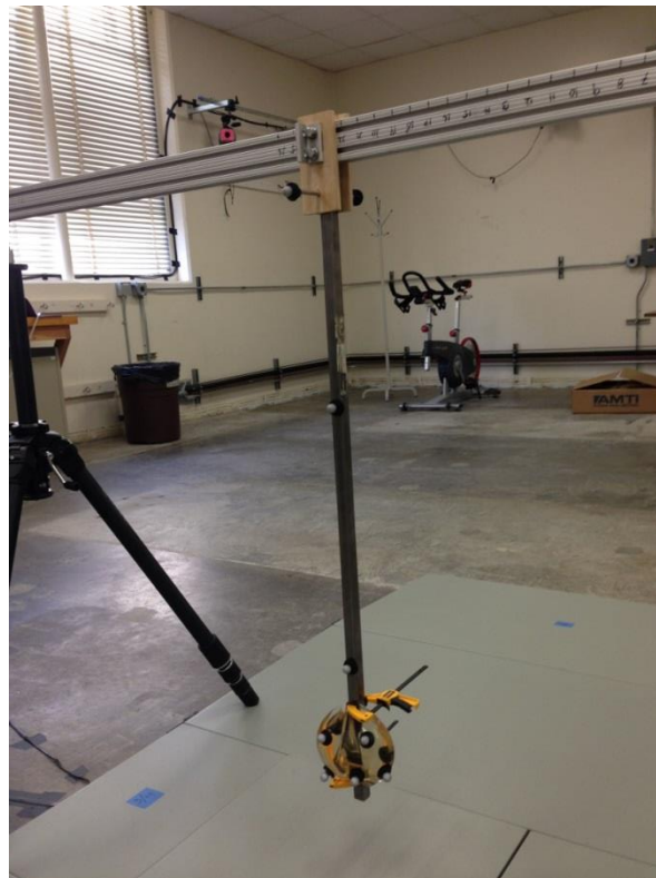
Figure 1. Pendulum apparatus fitted with implant and markers
