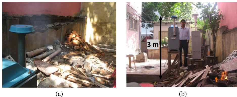
FIGURE 3 (a) High-volume sampler set up at a distance of 2 m upwind of the emission sources (b) same as (a) but standard reference height for particle sampling indicated
