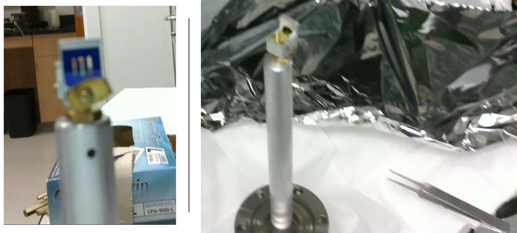
Figure D.2: Preparation Image of Gold Surface and Grating in Mount. Left: View of nanofabricated grating. Right: View of entire feedthrough (without the external translation stage and wobble mount)
