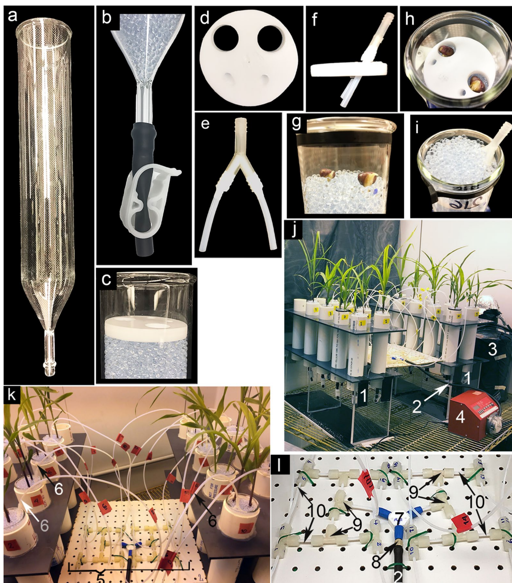
Fig. 1 Glass Bead semi-hydroponic system. a Glass tube. b Drain glass tube connected to 3 cm Viton tubing and closed with an acetal clamp. c Top of the glass tube filled with glass beads covered with a Teflon lid. d Details of the Teflon lid showing the four perforations. e “Y connector” attached to 4 cm Teflon tubing and sealed with Teflon tape. f “Y connector” inserted in the Teflon lid, showing the diagonal angle to water the plants. g Germinated seeds placed on top of the glass beads. h Planted seeds covered by the Teflon lid after planting. i Glass tube with planted seeds covered by glass beads and with the “Y connector” inserted. j Plants growing in the glass tubes in a growth chamber (1. Rack tubes, 2. Viton line, 3. Glass carboy containing Hoagland solution for watering plants. 4. Peristaltic pump). k Details of the watering system (5. Branched pipe 2 × 8, 6. Outlet lines inserted in the “Y connectors”). l Details of the branched pipe (7. 3-way connector, 8. Barbed adaptor, 9. Compression fittings, 10. Teflon tubing connecting the compression fittings)
