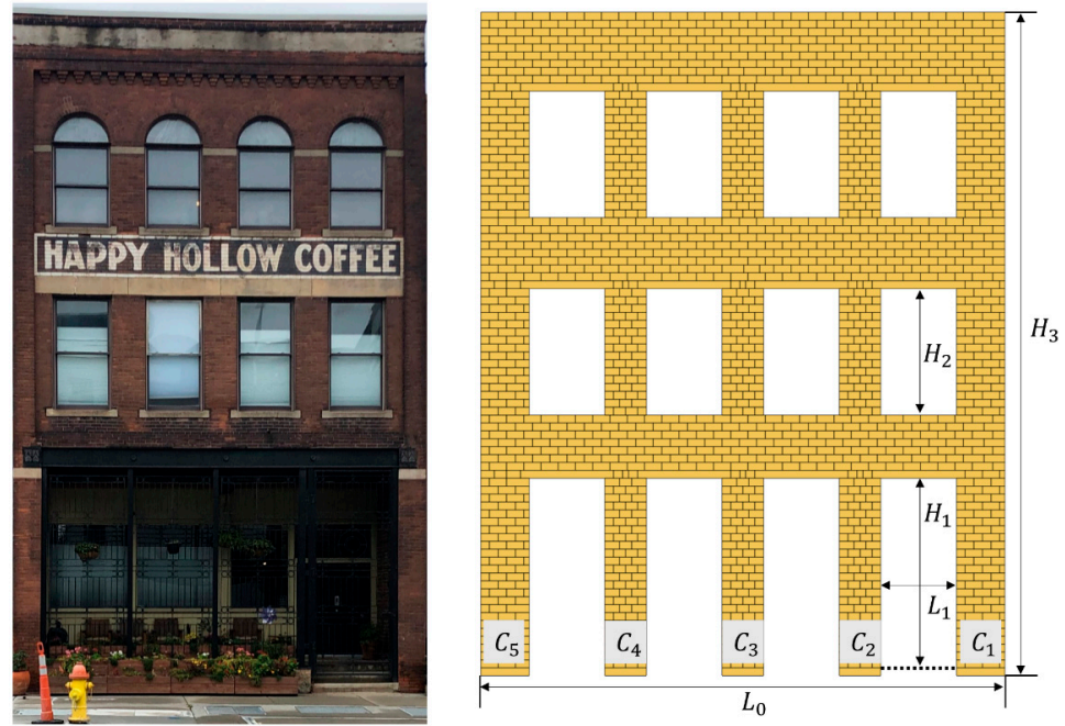
Figure 6. Historical building (left) and computational model (right); Dimensions: H_1 : 2.85, H_2 : 1.9, H_3 : 10, L_0 : 8, L_1 : 1.15—Dimensions are in meters, and columns are denoted as C_{i=1:5} .
