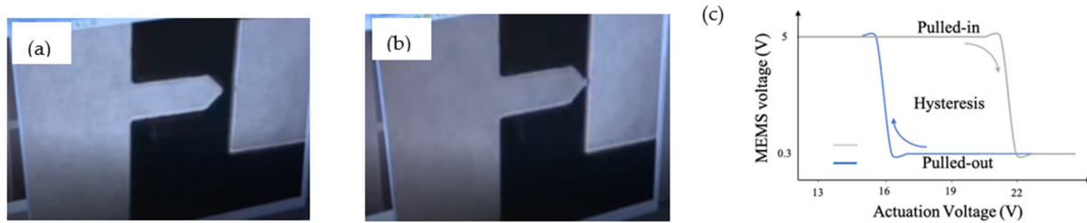
Figure 13. Pull out (a) and pull in (b) images for MEMS 3. (c) A sample hysteresis plot.
