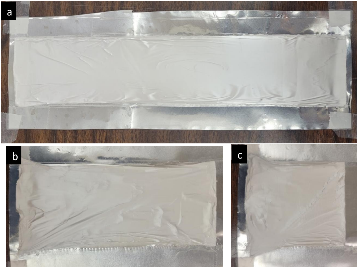
Figure B.2: Aligned PAN NF mats. (top) as-spun. (bottom left) folded over once to create a [0_2] layup. (bottom right) folded over twice to create a [0_4] layup. The fiber direction is horizontal.
