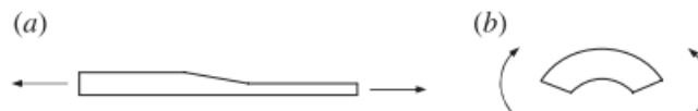
Figure 2.14: Features prone to delamination owing to geometry: (a) taper and (b) curved section in bending. 33
