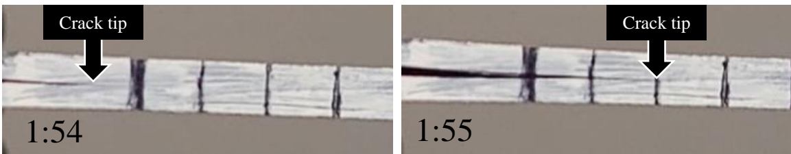
Figure 3.24: Unstable mode I crack propagation in a pristine carbon/epoxy specimen.
