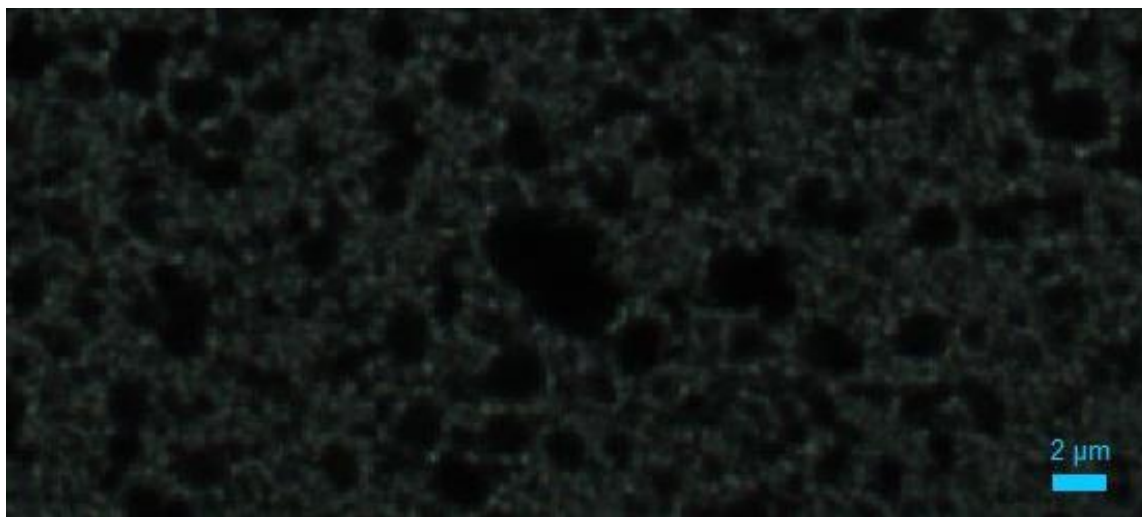
Figure D.3.1.3: Optical microscope image of the 10wt% PAN + 1% (wt% of PAN) GNR in DMF after sonication and evaporation of DMF solvent.
