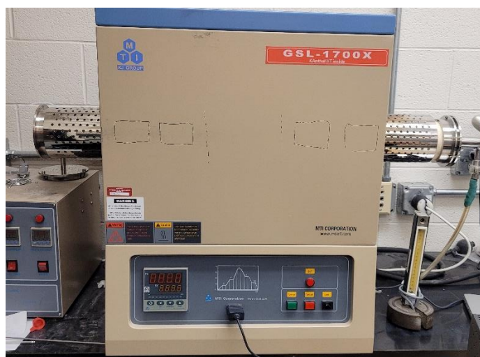
Figure B.1: MTI GSL-1700X tube furnace in which nanofibers were carbonized.
