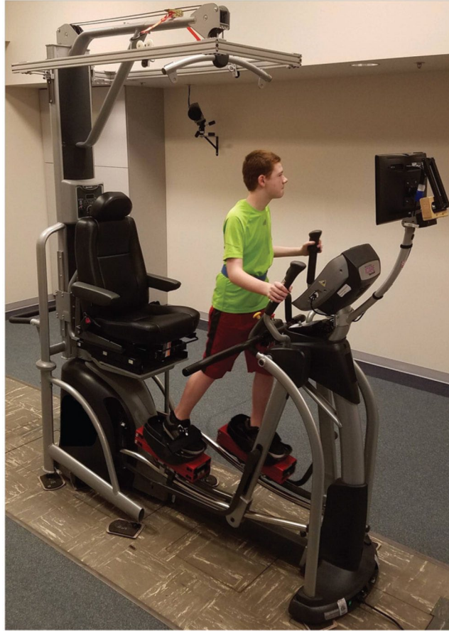
Figure 1. The motor-assisted elliptical device ICARE in use by our participant (photograph obtained with parental consent).
