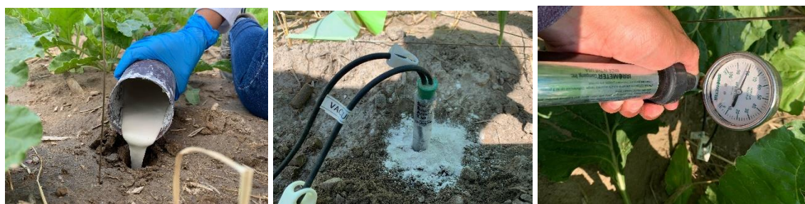
Figure 2.1 Installation and testing using a vacuum pump of the lysimeters used in this experiment.
