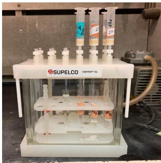
Figure 2.4 Visiprep™ SPE Vacuum Manifold holding the MDL and LRB samples during the elution process.
