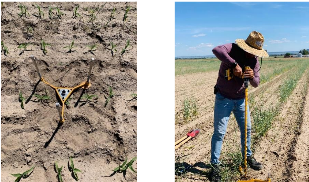
Figure 1.6 A special auger was used to drill holes for soil moisture sensors at 120 cm depth.
