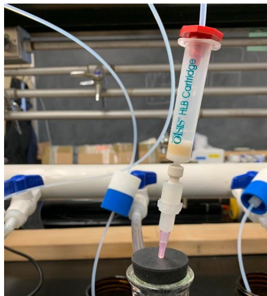
Figure 2.3 Sample extraction process using OASIS HLB 200mg/6cc solid phase extraction cartridges.
