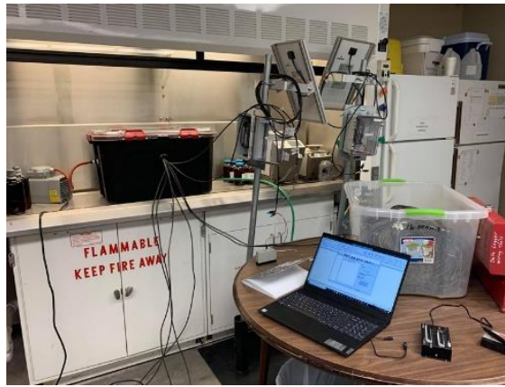
Figure 1.5 Oxygen sensors calibration prior their installation in field.
