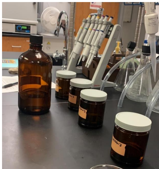
Figure 2.2 Amber jars containing 50 grams (around 50 mL) of DDI water, 10 mL of McIlvain-EDTA buffer solution and Analyte/Surrogate Spikes.
