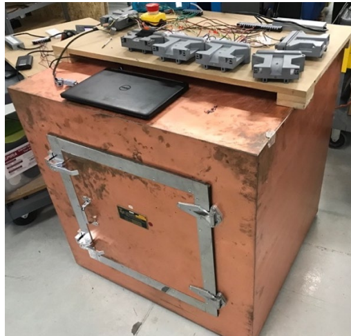
Figure 5.7: Copper radio frequency blocking box used to perform tests on STAVE
