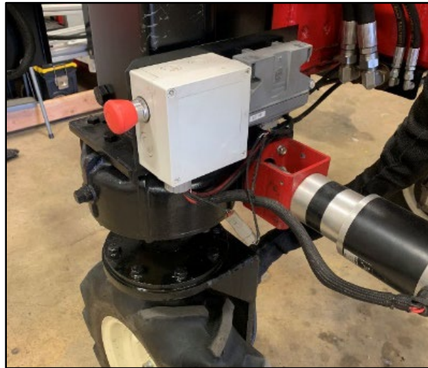
Figure 4.3: E-stop button on a corner of Flex-Ro
