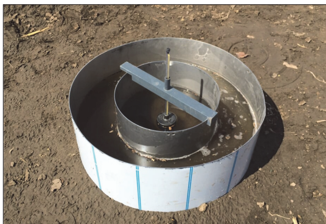
Figure 3. Double-ring infiltrometer used to measure saturated hydraulic conductivity ( K_s ) of different treatments in this research. This picture was taken when measuring K_s in a bare soil plot.
