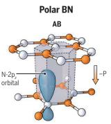
AB or BA stacking is more stable than AA. The vertical alignment of the B and N atoms distorts the N-2p\_z orbital.
