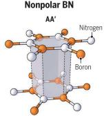
AA' layer stacking, the bulk form of h-BN. Layers are stacked at a 180° angle with respect to each other, making h-BN nonpolar.
