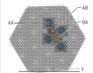
Adding a small-angle (Y) twist between *h*-BN sheets creates relatively large AA regions separated by AB and BA domains.
