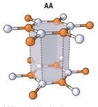
AA layer stacking has layers related by mirror symmetry, but this configuration is not stable.
