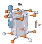
The AB or BA stacking creates an out-of-plane electric dipole pointing down (-P) or up (+P).
