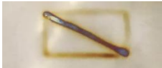
Figure 5. Effect of CNC interpolation on laser processing of thin sheets.
