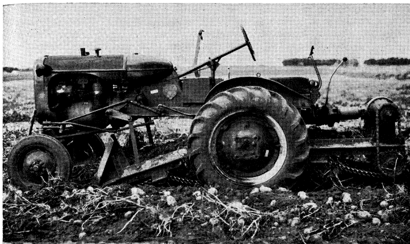
Custom-built level-bed potato digger mounted under tractor and used for harvesting outstate tests. It can be turned sharply for use in small plots. The whole assembly is easily loaded on a truck.
