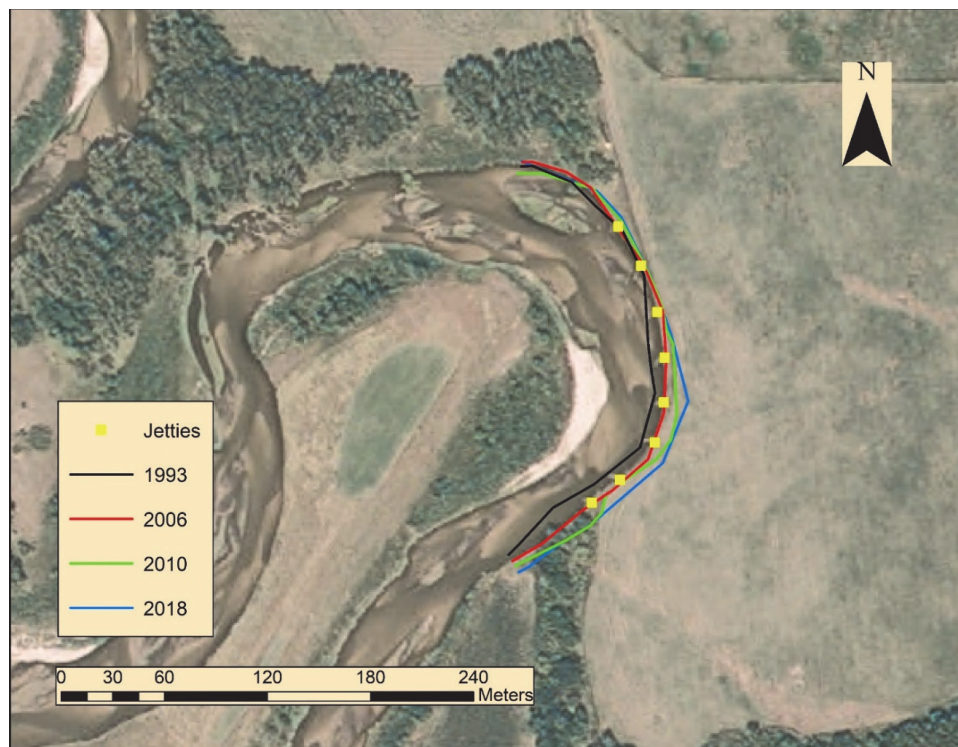
Figure 4. At site 15, the jetties installed prior to 2006 were no longer in place during our site visit in 2019, resulting in continued streambank retreat from 2006 to the present.
