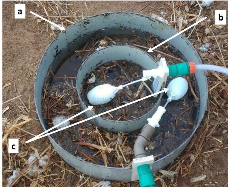
Fig. 3. Example of infiltration test performed on cropped areas in UAS region. System description: a) Outer ring, b) Inner ring, c) Floats valves.
