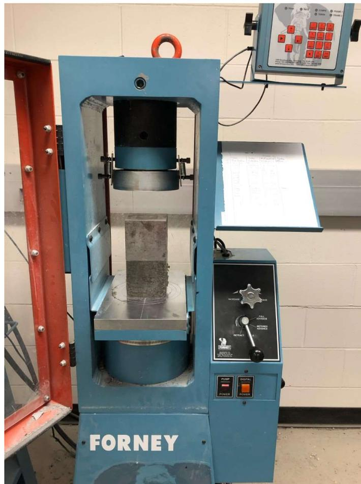
**Figure 3.7.** Compressive strength apparatus
