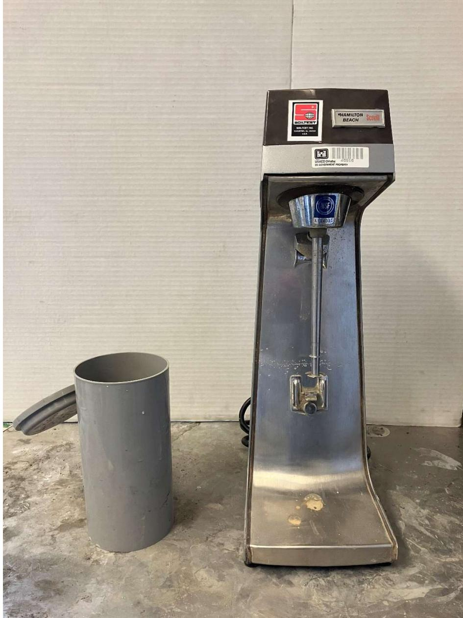
**Figure 3.2.** Higher shear blender and cylinder used to pre-blend nanomaterial
