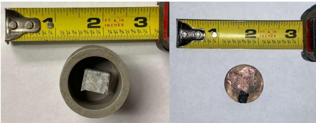
**Figure 3.9.** SEM Samples before and after resin casting
