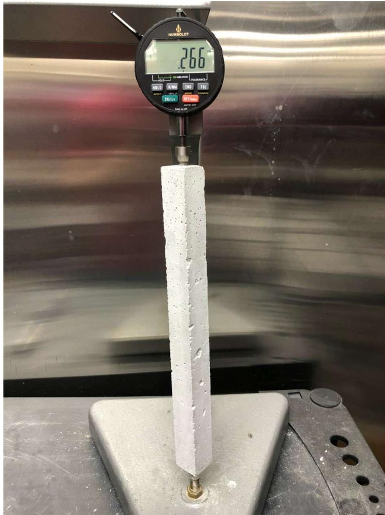
**Figure 3.8.** Drying shrinkage testing apparatus
