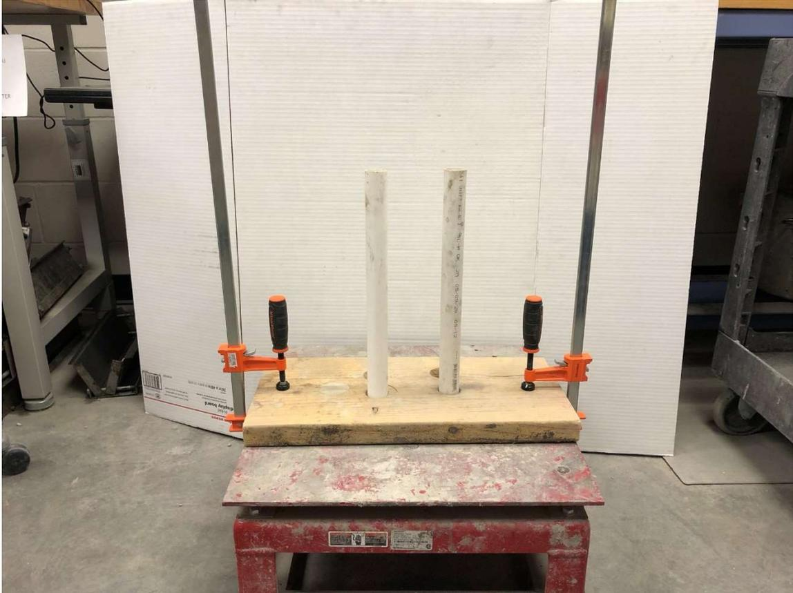
**Figure 3.5.** Support Frame for Casting Autogenous Shrinkage Samples
