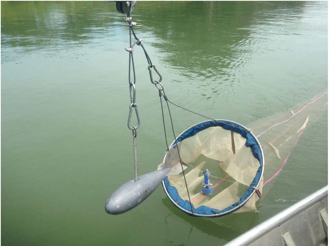
Figure 2-1. Drift net used for larval fish sampling. Net is equipped with a flow meter and 45 kg bomb weight to hold it in the current.
