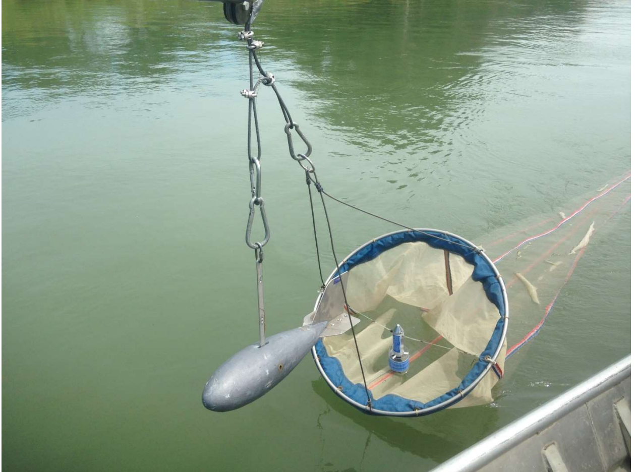
Figure 3-2. Drift net used for benthic larval fish sampling. Net is equipped with a flow meter and 45 kg bomb weight to hold it in the current.
