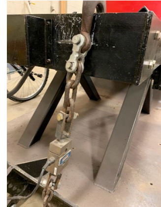
Figure 7: Photo of the current load cell setup used by the Quarter-scale team.
