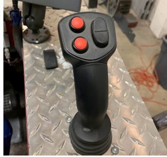
Figure 5: Image of physical JS6000 Danfoss Joystick on pulling sled. The red buttons actuate the lift cylinder and the toggle button moves the weight box. Motion on the Y-axis propels the sled.
