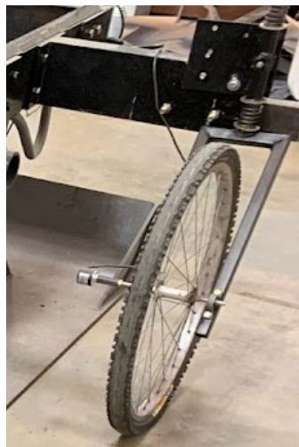
Figure 11: Image of "fifth wheel" bike tire and suspended mount implemented to employ use of the rotary encoder.
