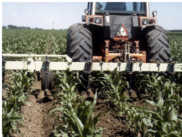
Figure 10.4. Forming furrows for furrow irrigation.
