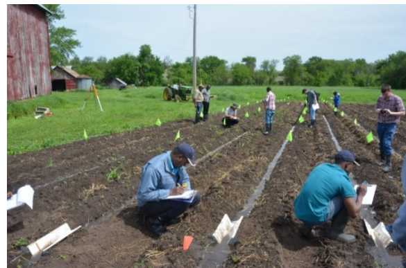
Figure 10.8. Students measuring stream size, advance, recession, and runoff in a furrow irrigation system. (Photo courtesy of Laszlo Hayde, IHE Delft Institute for Water Education.)
