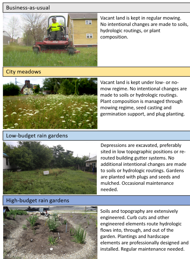
Fig. 2. Four scenarios—Business-as-usual, City meadows, Low-budget rain gardens, and High-budget rain gardens—were schemed for a vacant land management program intended to identify desirable green infrastructure strategies in Cleveland.
