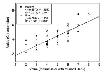
**FIGURE 5** Relationship between value measured with Munsell book and chromameter-measured value for readings taken in the early morning and at noon under sunny conditions. Visual color data were collected by the four individuals with the highest overall accuracy in the study and include both moist and dry colors
