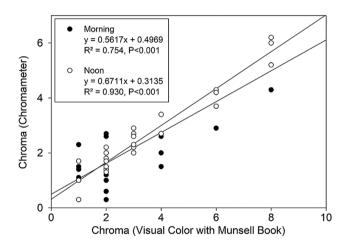
**FIGURE 6** Relationship between chroma measured with Munsell book and chromameter-measured chroma for readings taken in the early morning and at noon under sunny conditions. Visual color data were collected by the four individuals with the highest overall accuracy in the study and include both moist and dry colors
