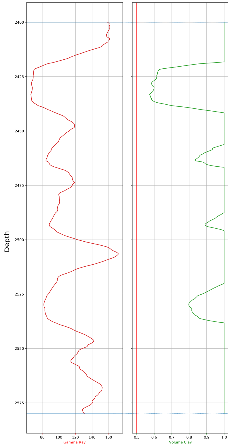
Figure 40: Depth versus GR and VolClay from the well Otates 14.
