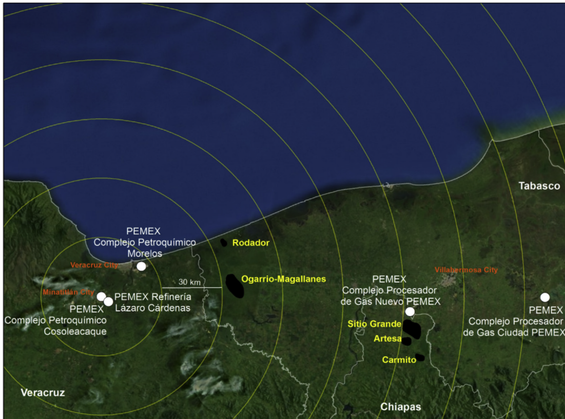
Figure 2.5: Industrial CO 2 sources (> 0.5 Mtpa) located near Cinco Presidentes oil fields. Taken from Lacy et al. (2013).
