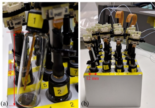
Fig. 3. Sensors in vials prepared for electrolyte submersion, (a) two thermistors populated per PCB, (b) vials placed in block (constant 25 °C).
